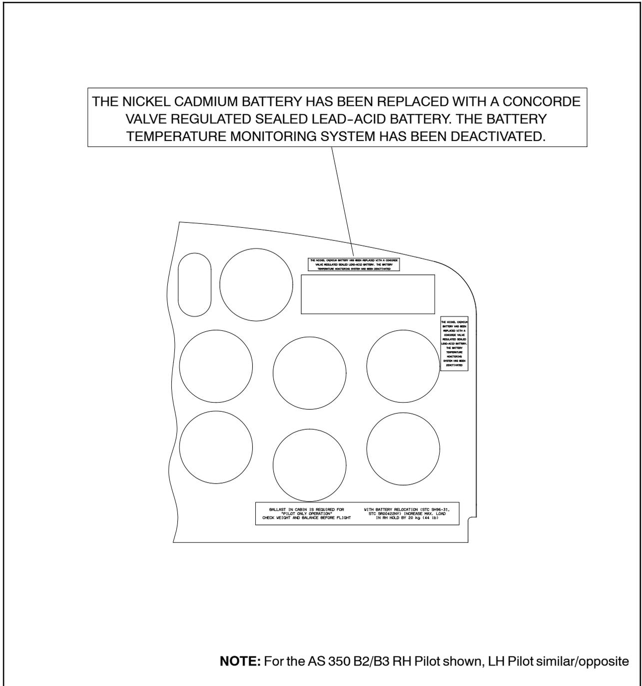
Figure 22 Placard location on typical AS 350 Instrument Panel (Lead-Acid Battery only) RH Pilot configuration
