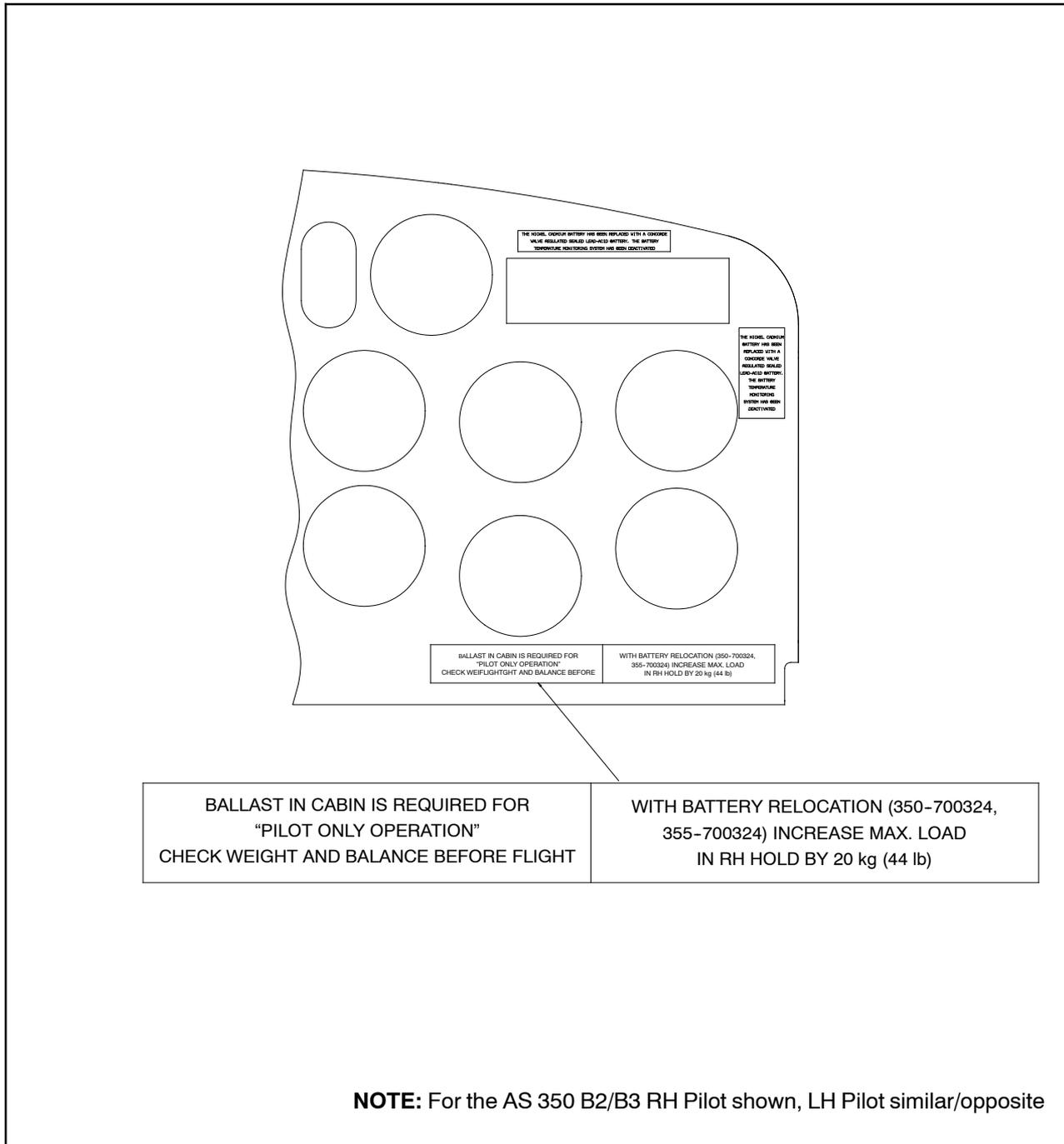
Figure 23 Placard location on typical AS 350 Instrument Panel, RH Pilot configuration
