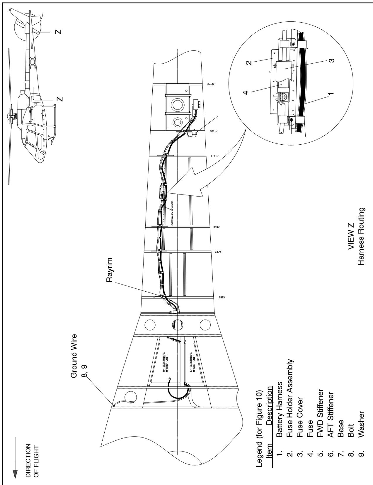
Figure 10 AS 355 Harness Routing - Tail Boom
