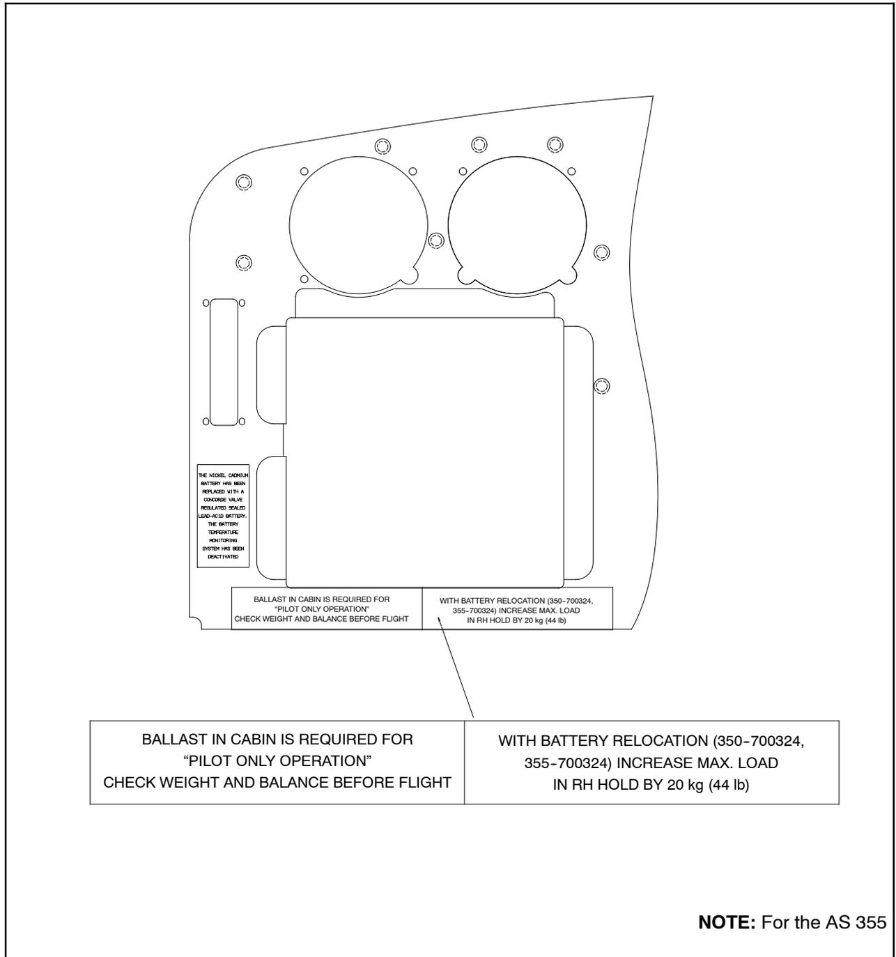
Figure 24 Placard location on typical AS 355 Instrument Panel
