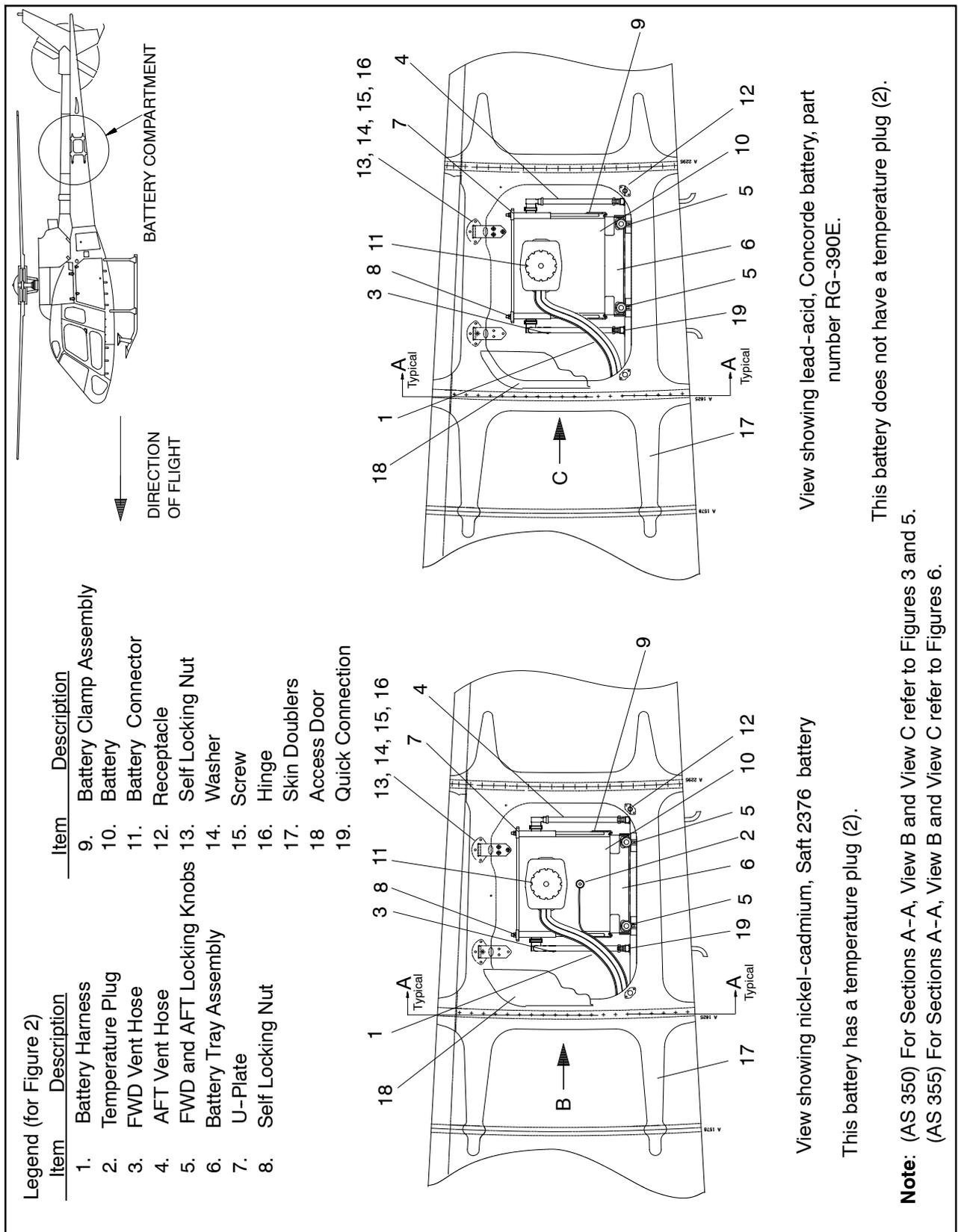
Figure 2 AS 350 and AS 355 Battery Compartment (main views)
