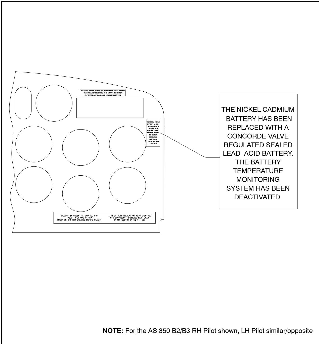
Figure 21 Placard location on typical AS 350 Instrument Panel for RH Pilot Configuration (Lead-Acid Battery only)
