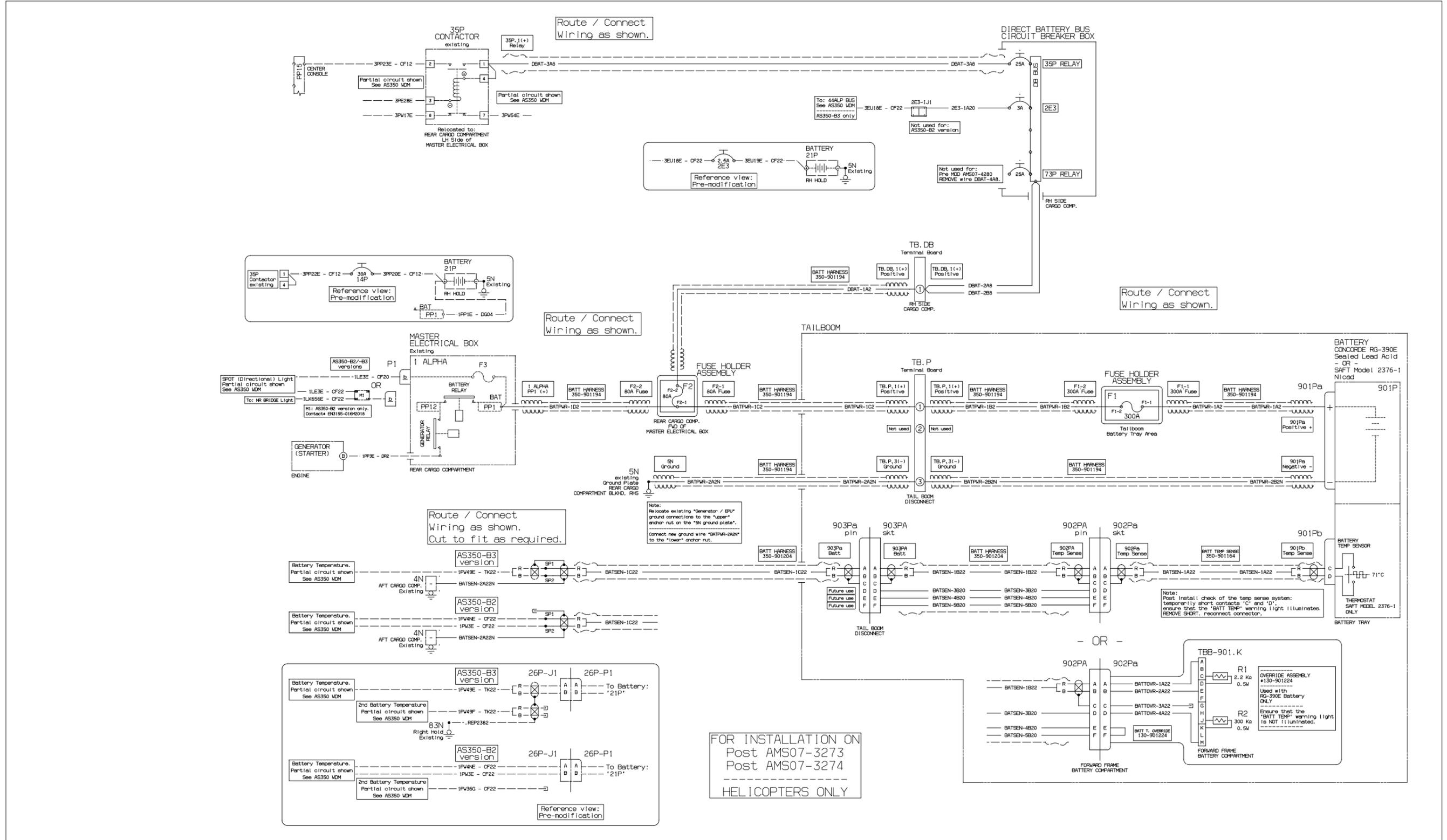
Figure 15 AS 350 Battery Relocation, Wiring Diagram
