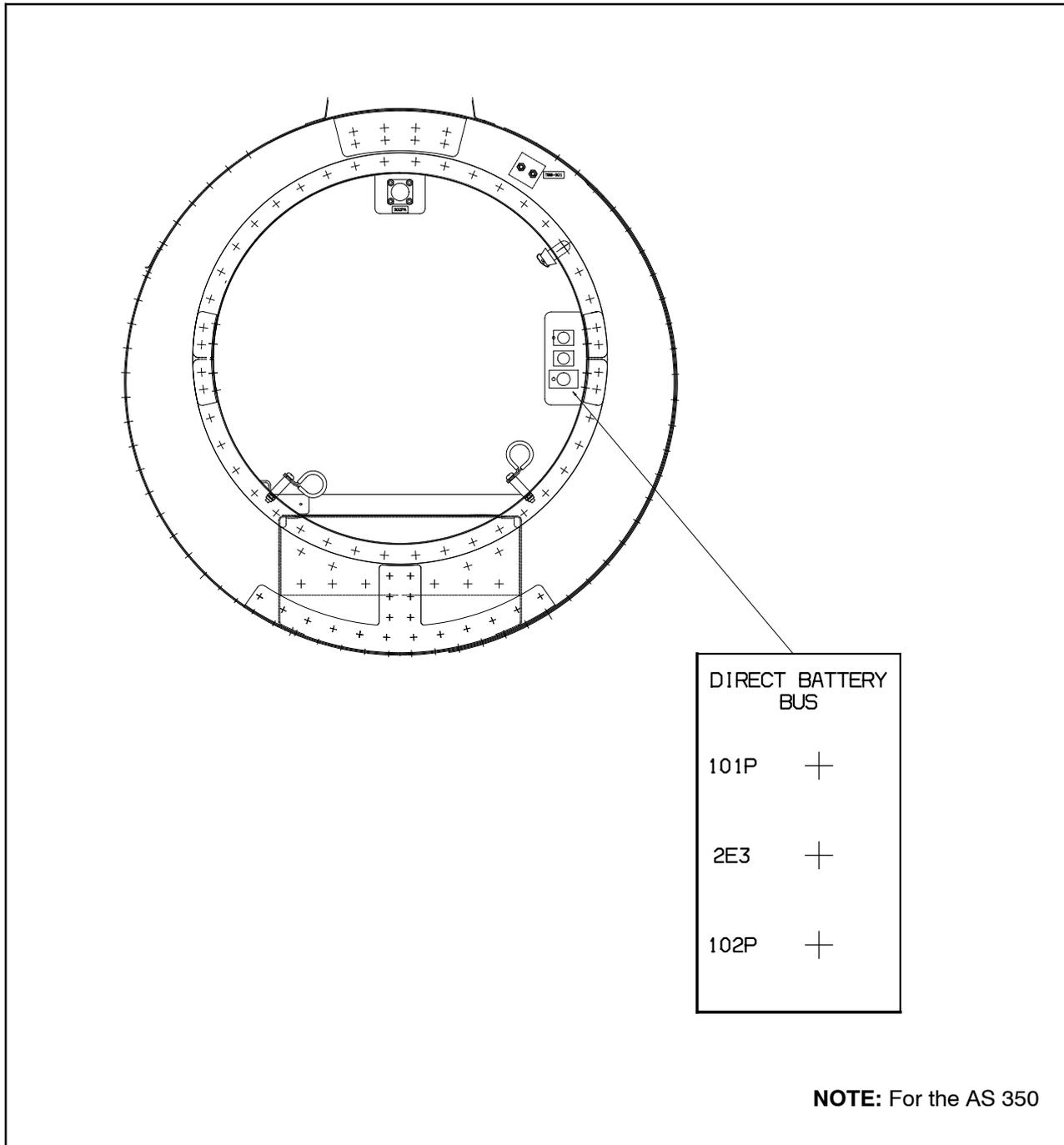
Figure 27 Marking location on the AS 350 circuit breaker bracket at STN A1825
