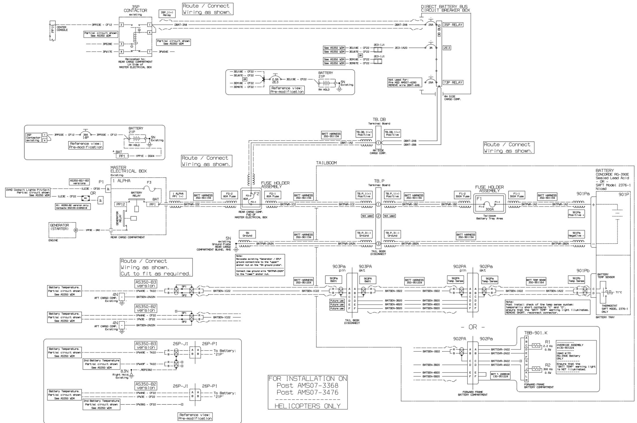
Figure 18 AS 350 Battery Relocation, Wiring Diagram (continued)
