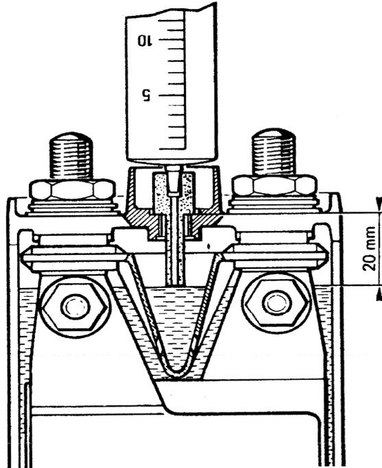
FILLING PRINCIPLE WITH A CALIBRATED ENDPiece SYRINGE
