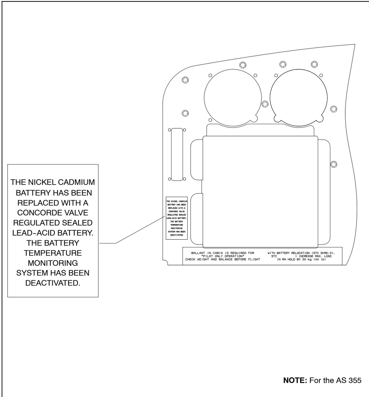
Figure 25 Placard location on typical AS 355 Instrument Panel (Lead-Acid Battery only)
