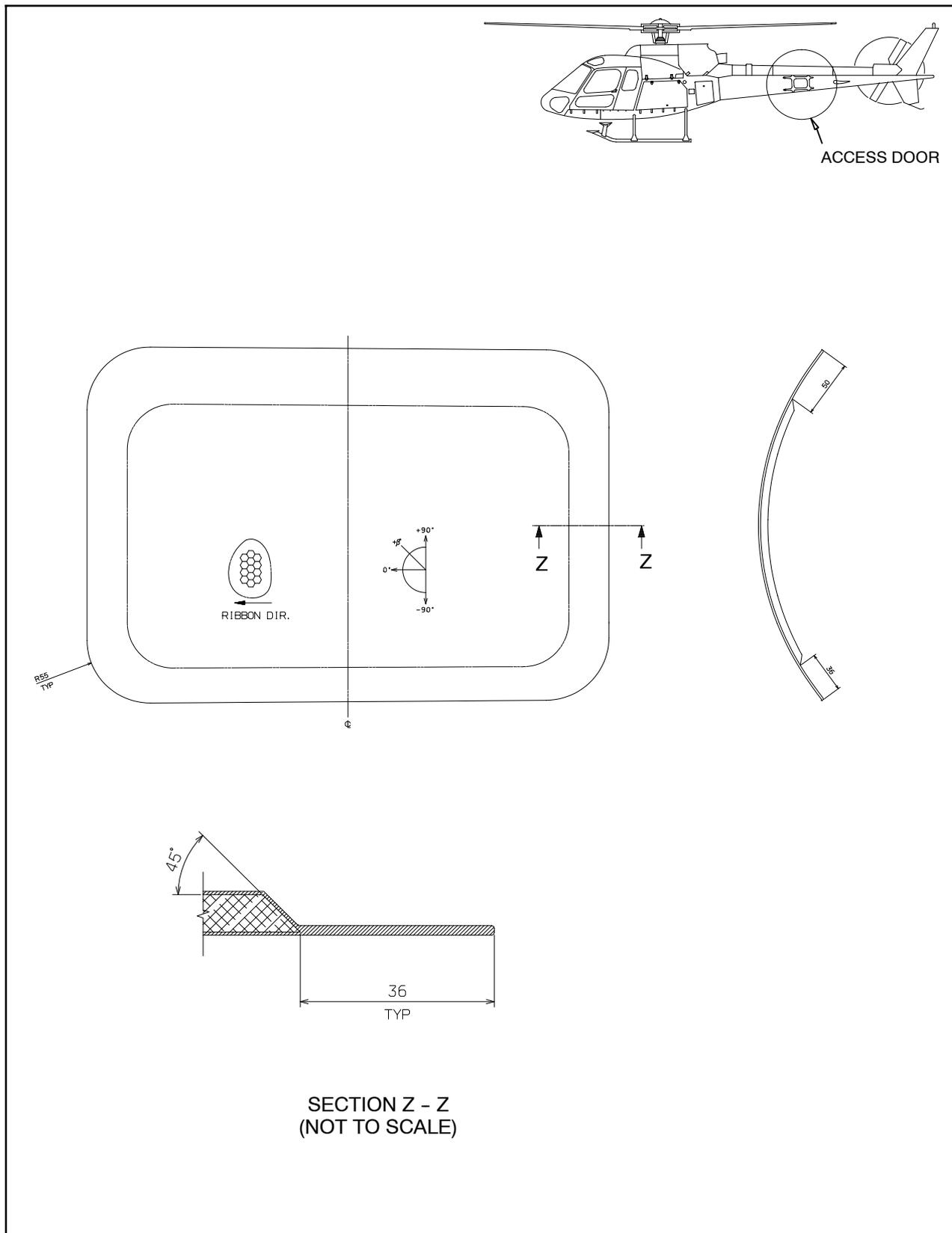
Figure 14 Access Door - Composite Layup
