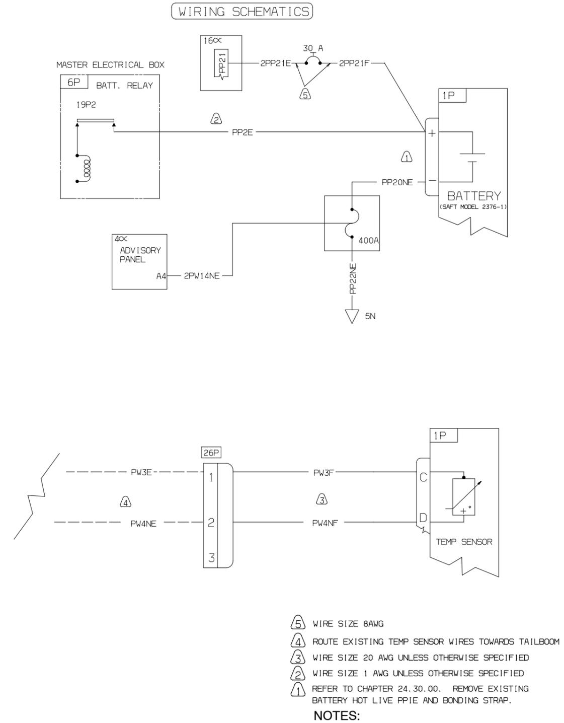
Figure 20 AS 355 Battery Relocation, Wiring Diagram
