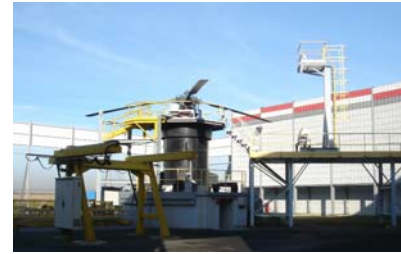
Dynamic tower track and balance test stand in La Courneuve, France
