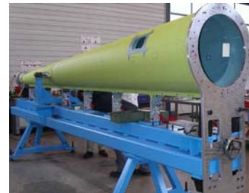
Tailboom repair jig
