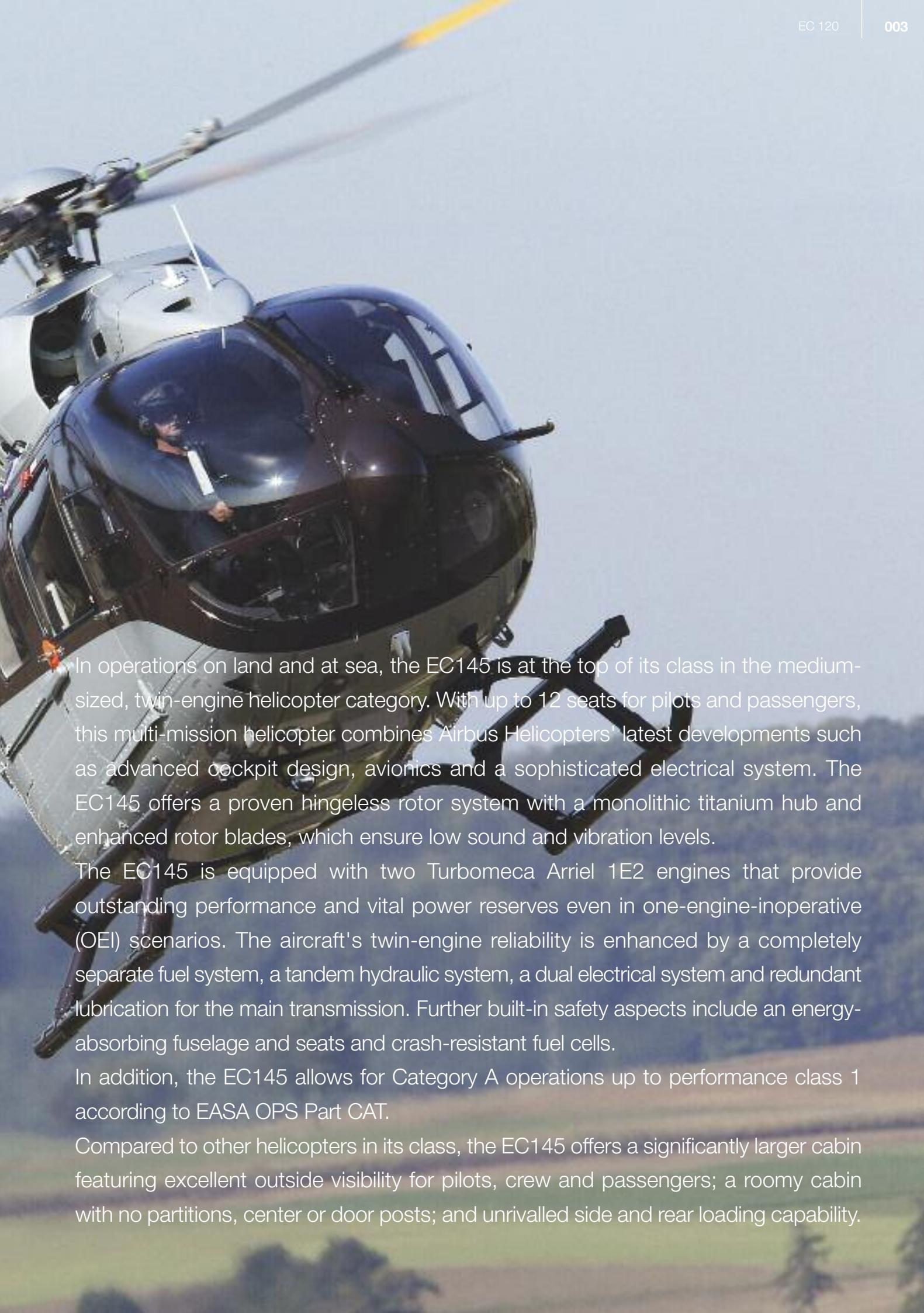
In operations on land and at sea, the EC145 is at the top of its class in the medium-sized, twin-engine helicopter category. With up to 12 seats for pilots and passengers, this multi-mission helicopter combines Airbus Helicopters' latest developments such as advanced cockpit design, avionics and a sophisticated electrical system. The EC145 offers a proven hingeless rotor system with a monolithic titanium hub and enhanced rotor blades, which ensure low sound and vibration levels.
