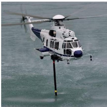
Pump operable in very shallow water, filling in 90 seconds
