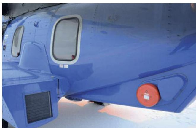
ADELT (Automatically Deployable Emergency Locator Transmitter for Helicopters)
