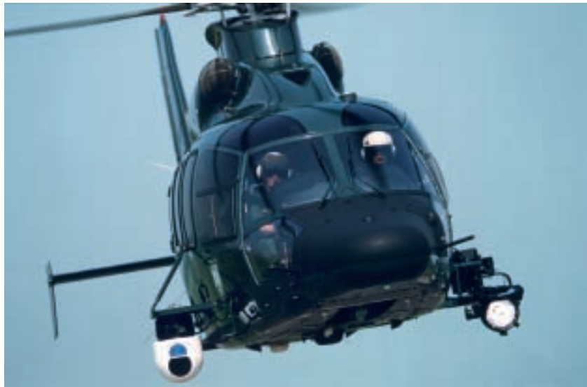
Upper and lower cable cutters for wire-strike protection
