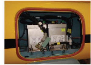
EC130 SECOND BATTERY INSTALLATION
