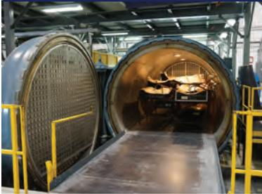
Composite Curing through autoclaves, ovens & platen press
