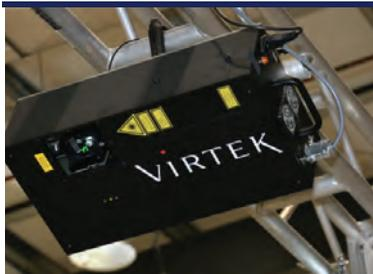
Laser system for ply placement accuracy
