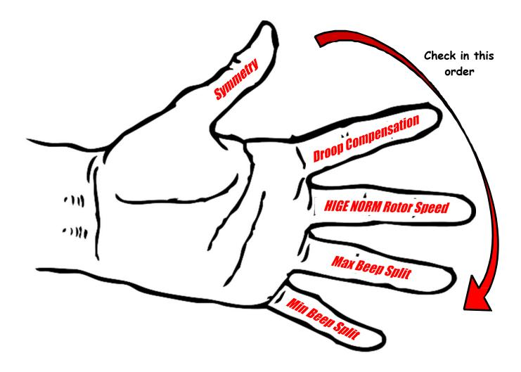
If these 5 items are within limits and there are no deficiencies with airframe or engine components, then VARTOMS will function properly
